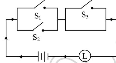
28. Draw the simplified circuit of the following switching circuit.
