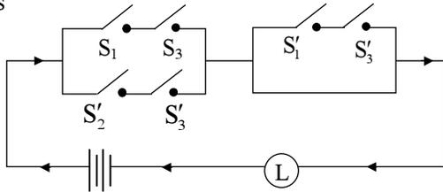
25. Simplify the following circuits so that the new circuit has minimum number of switches. Also draw the simplified circuit.
